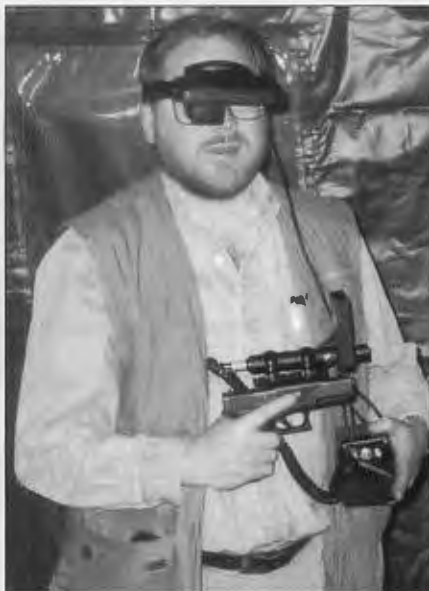
Norquist tests and evaluates a thermal-imaging scope that enables a shooter to see around corners.
